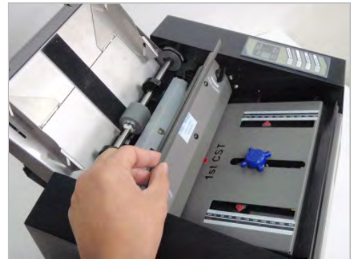
[Open the cover and remove the jam]
