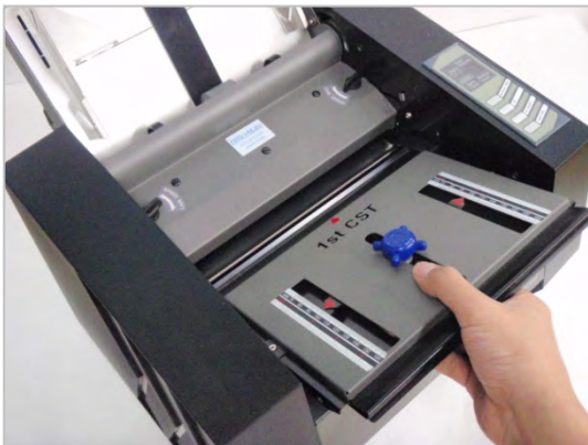
[Pic.1 : 1 st Cassette Assemble]
